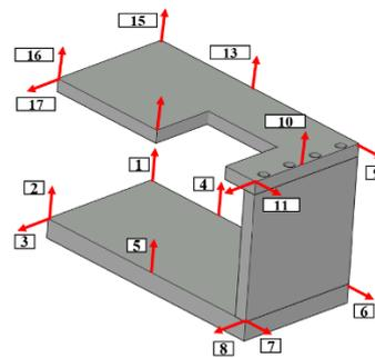
(b) Placement of accelerometers
