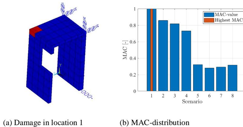
Figure 10: MAC-SBDA on damage location 1
