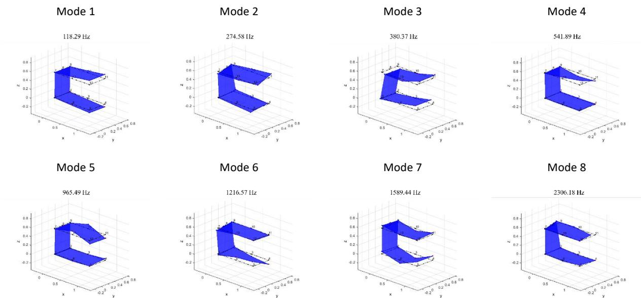
Figure 6: Experimental modeshapes for the first 8 modes
