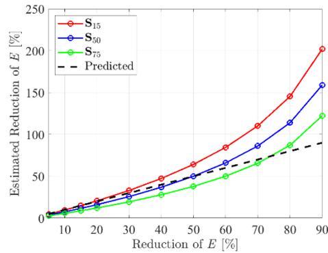
Figure 16: Influence of sensitivity matrix when simulation damages between 0% and 90% on location 1
