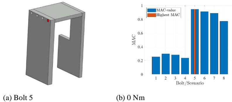
Figure 20: MAC-distribution for damage on bolt 5
