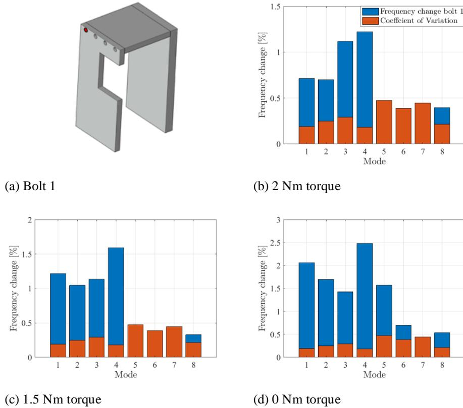
Figure 17: Frequency changes for damage for bolt 1 along with the coefficient of variance
