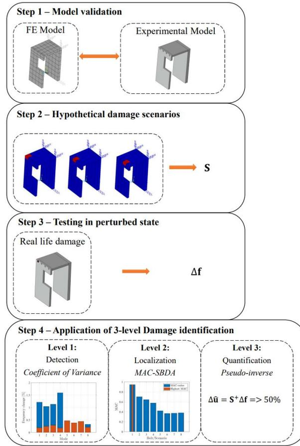
Figure 1: The four steps to perform the 3-level damage identification
