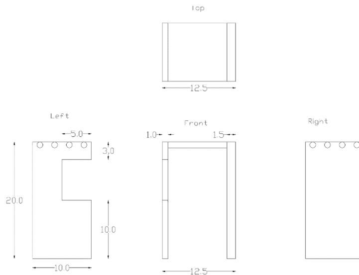
*Figure 2: Dimensions of laboratory specimen*
