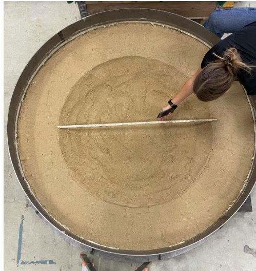
Figure 5 – Steel container with compacted sand excavated for the pocket.
