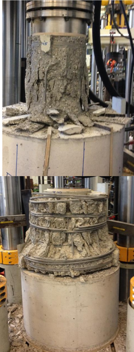
Figure 17: Crushing of piston before yielding of stirrups in sleeve of specimen 5-H-D (left) and damages of sleeve in specimen 6-H-W after ca. 480 mm piston displacement (right)
