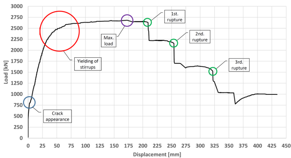
Figure 12: Load vs. piston displacement for specimen 1-L-D (Yield plateau replaced by Yielding of stirrups)
