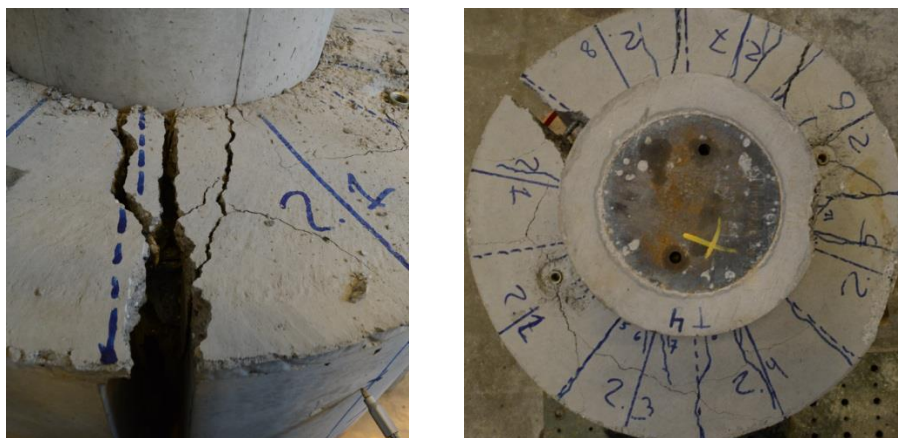
Figure 15: Crack patterns and location of stirrup rupture in sleeve, top view of specimen 2-L-D.
