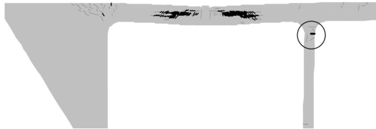
Figure 12. Crack pattern at peak load  $P=10.5$  MN. Cracks larger than 0.5 mm. Taken from [3].
